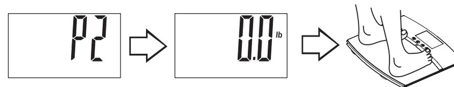
Stand still while the scale measures your weight. Your weight will display for 2 seconds, and then the scale will begin to estimate your body composition. The screen shows a moving zeros pattern (“0000”) while estimating. Continue to stand still on the scale.
